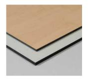
EGGER compact laminates Flammex Euroclass B are flame-retardant compact laminates according to EN 438-4, respectively EN 438-8 with a black core based on curable resins. They have a multilayer structure and consist of melamine resin impregnated decorative paper and multiple layers of soda kraft paper impregnated with phenolic resins, which are laminated under high pressure and heat.
